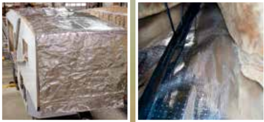
Radiant shield Thermo-foil – R-38
