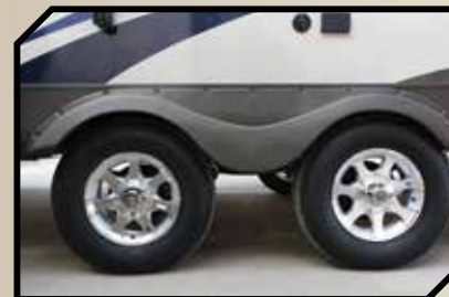
WIDE TRACK SUSPENSION (TRAVEL TRAILERS ONLY) WITH ALUMINUM RIMS
